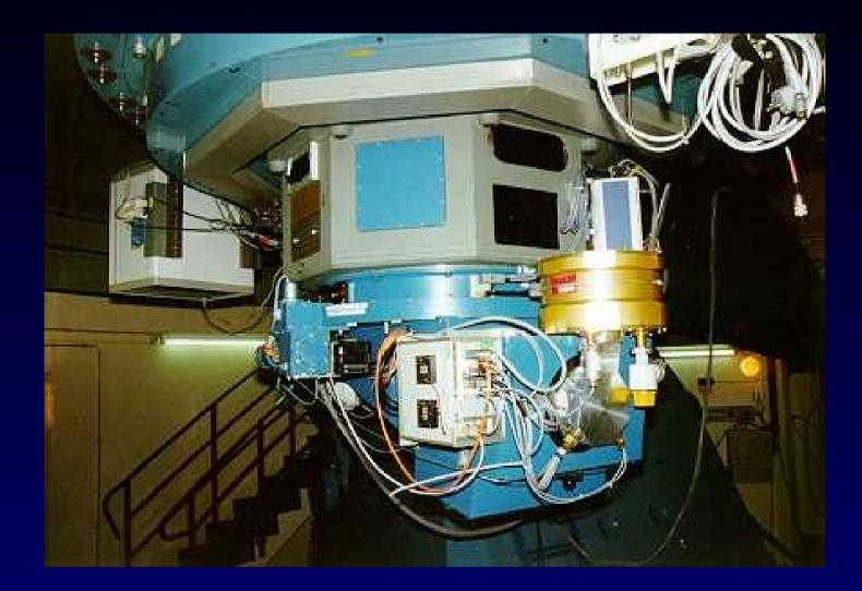
Camera CCD 2048x2048 (cut 4k) 13.5x13.5 arcmin filters U,B,V,R,I Halpha, Hbeta .... 3 groups of Czech astronomers
