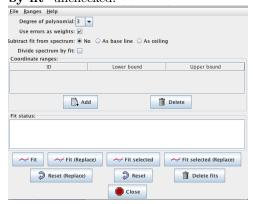
Click on **Add** and select several coordinate ranges where the spectrum is relatively flat, leave the strong peaks out. When you are ready, click on the **Fit** (**Replace**) button. The polynomial fit curve will be shown on the plot, and will be listed on the **Global list of spectra** in the main SPLAT-VO window.
